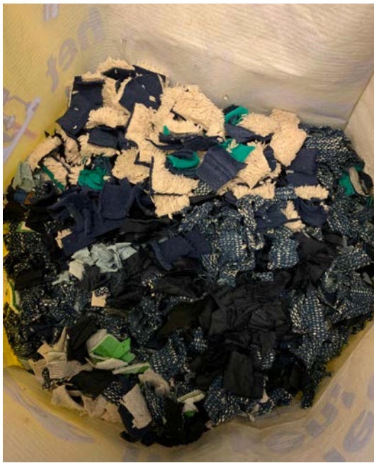
Figure 4. Sample of cuttings from the selected clothing items, cut into 1x1 cm pieces.
