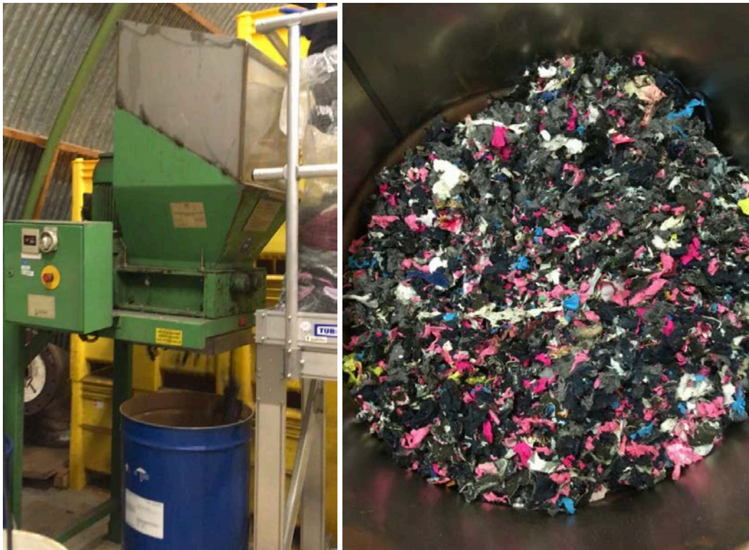
Figure 22. The shredding machine (left) and resulting shredded output (right).
