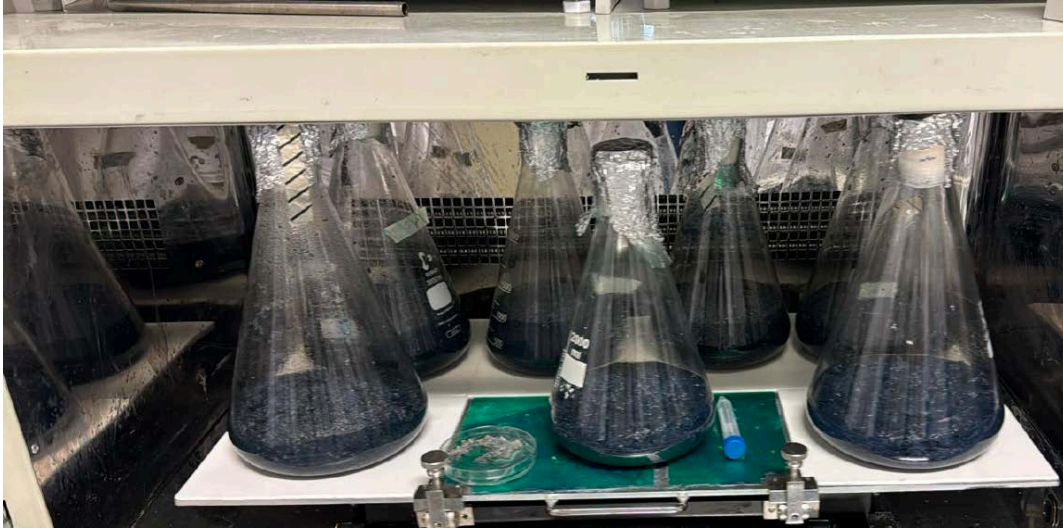
Figure 10. Enzymatic hydrolysis process (i.e. cellulose-to-glucose transformation) across multiple vessels.
