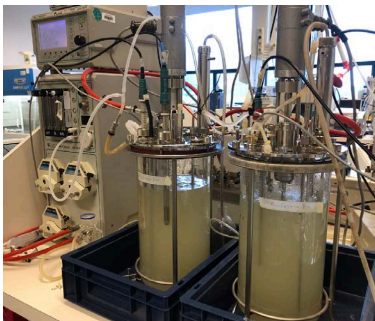
Figure 9. Fermentation of enzyme cocktail created for the purpose of textile degradation.
