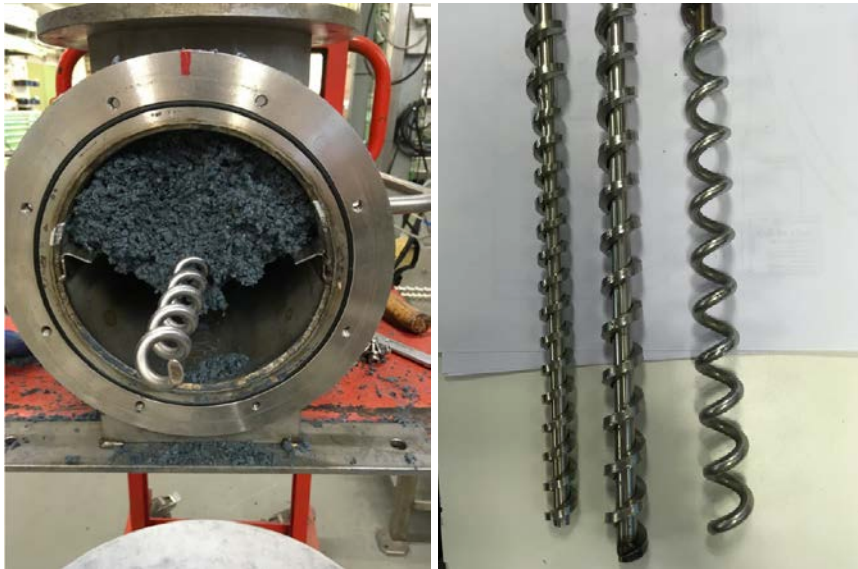
Figure 29. The blocked entrance in the feedstock bunker (left), three different feeding screws (right).
