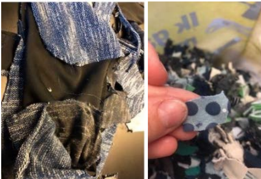
Figure 3. Sample of composite materials, or layered fabrics joined by adhesives, and textile with 'plastic' decorations.
