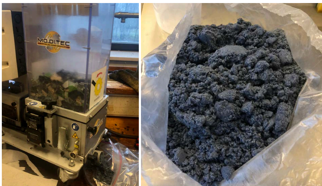
Figure 8. Textile cuttings being ground into smaller pieces.
