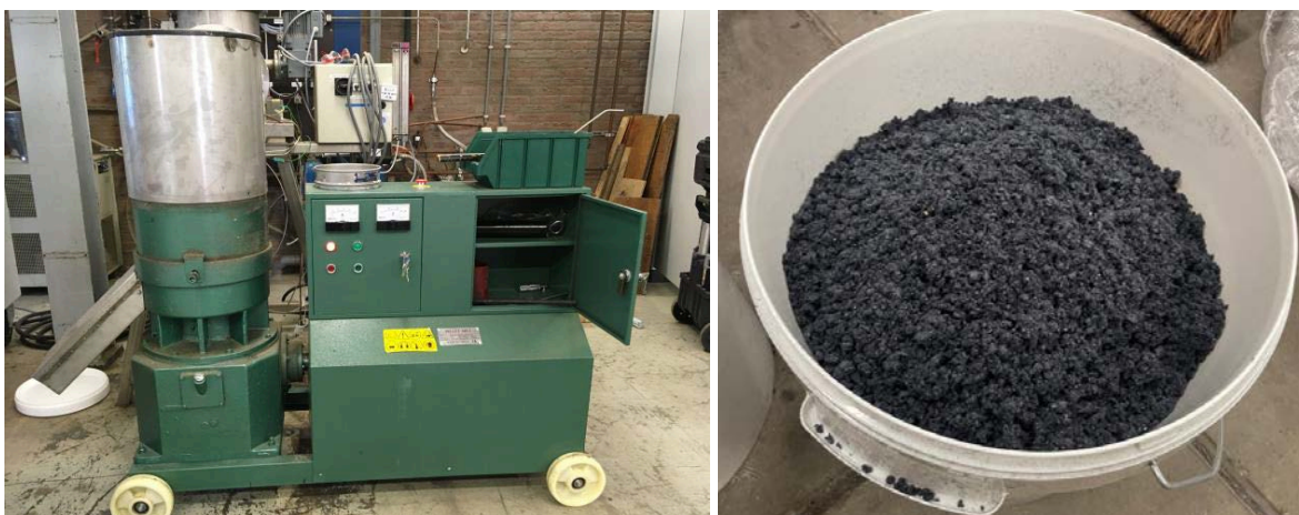
Figure 23. depicts the pelletising machine (left) and resulting shredded output (right).
