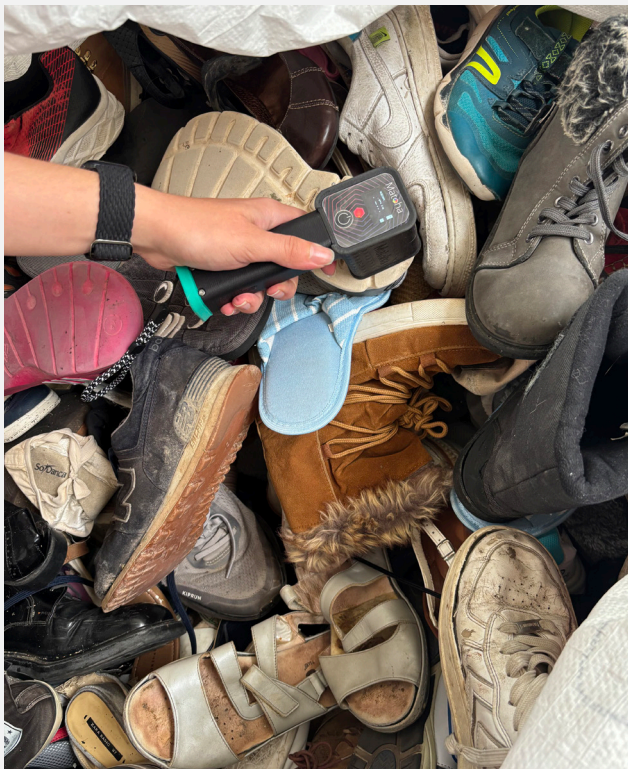
Figure 4: Matoha's ShoeTell to Identify Footwear Sole Material, set-up at CETIA
