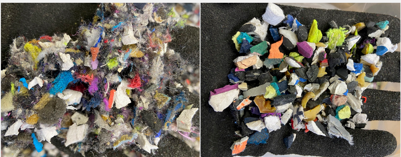
Figure 9: Shred and separated output at ELDAN Recycling, on the left, light fraction, and on the right, heavy fraction
